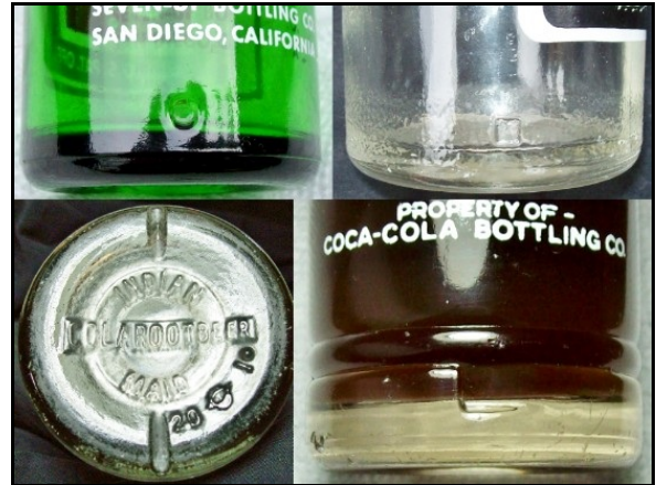
Figure 28 – Clockwise from top: Indexing dimple, button, ramp, and base slots
